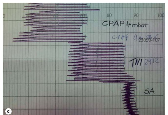
Fig. 1. a nHF device with thick nasal prong. b Setup for measurement of pressure changes, with nHF device (left), amplifier (lower right), Hämobox and pen recorder (upper right). c Example of pressure diagram. SA = Spontaneous breathing; TNI = nHF device; pressure amplitude = peak to trough; mean pressure increase = shift to the left.
