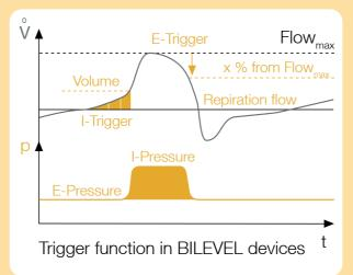
The BILEVEL devices offer two levels of pressure (I-pressure and E-pressure). The triggers which are separately adjustable for inspiration and expiration are particularly well suited to shallow breathing and effectively avoids undesirable selftriggering. The inspiration trigger controlled by volume and expiration trigger controlled by flow are adjustable in three settings.
