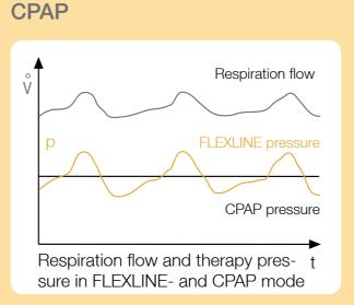
In the FLEXLINE mode the pressure adjusts proportionally to the individual respiration flow. This means an increase in pressure on inspiration and a reduction in pressure on expiration. This results in a particularly gentle therapy.
