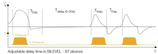
The BILEVEL devices offer two levels of pressure (I-pressure and E-pressure). The triggers which are separately adjustable for inspiration and expiration are particularly well suited to shallow breathing and effectively avoids undesirable selftriggering. The inspiration trigger controlled by volume and expiration trigger controlled by flow are adjustable
