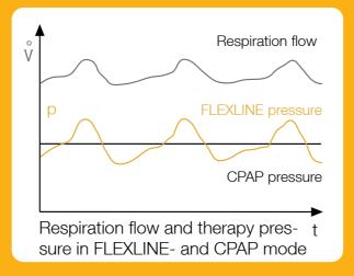
In the FLEXLINE mode the pressure adjusts proportionally to the individual respiration flow. This means an increase in pressure on inspiration and a reduction in pressure on expiration. This results in a particularly gentle therapy.
