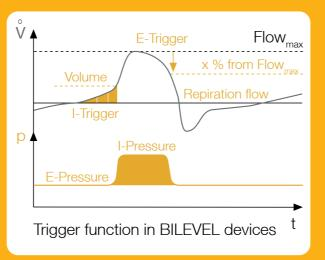
The BILEVEL devices offer two levels of pressure (I-pressure and E-pressure). The triggers which are separately adjustable for inspiration and expiration are particularly well suited to shallow breathing and effectively avoids undesirable selftriggering. The inspiration trigger controlled by volume and expiration trigger controlled by flow are adjustable in three settings.
